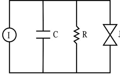
Figure 18.1: Resistively shunted Josephson junction. The capacitance  $C$  is the capacitance of the junction.
